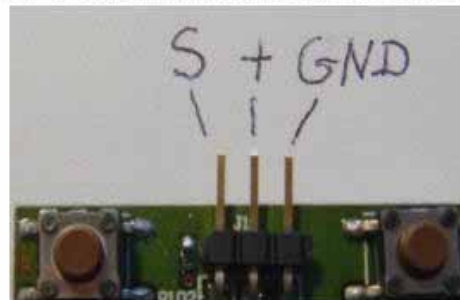
The GPS Unit with the 3 important connectors
