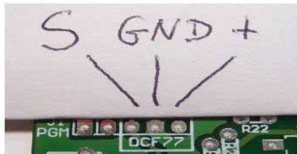
The clock pcb with the important connectors
